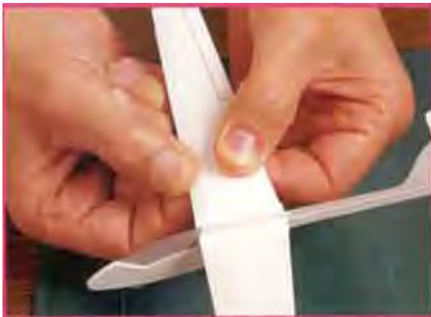
Figure 11-7-5 Adjusting Wing Curvature (Camber)
